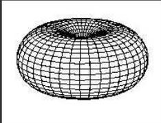
Dipole (the fundamental element of virtually all traditional industry antennas) Gain = 2.15dBi or 0dBd
