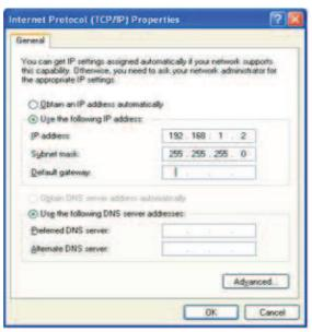
While most devices automatically detect DNS, you can set the DNS to the settings shown on the Dashboard screen of the modem user interface. Default Gateway of computer has to = the IPAddress of the modem Preffered DNS servers = modem DNS Servers #1 Alternate DNS server = modem DNS Servers #2.
