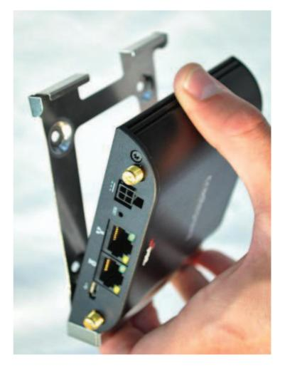
3) Press the router down firmly, then push it inside the bracket. It should latch.
