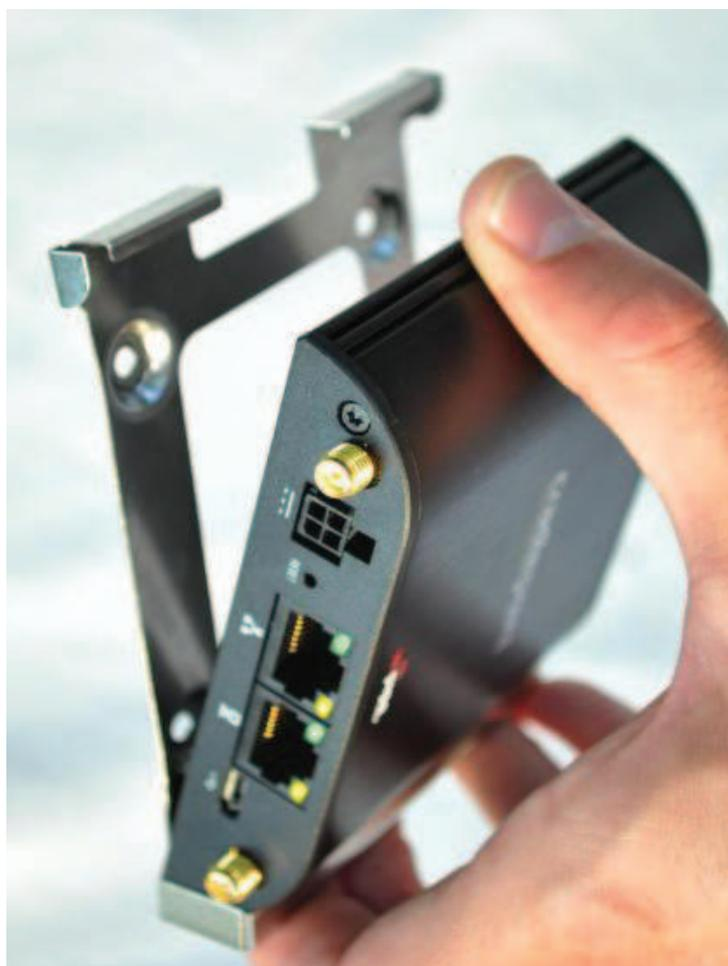
3) Press the router down firmly, then push it inside the bracket. It should latch.
