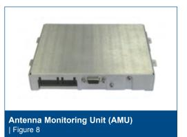
Note 1: The DC resistance of the antenna together with the cable connected to the SCU-4 should be less than or equal to 1 kilo ohm for the AMU to sense the antennas successfully. Note 2: AMU may not sense antenna if splitters are used between the connected antenna and the SCU-4.
