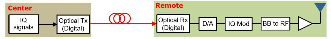
Long latency; synchronization and jitter issues; high speed D/A (high cost); high power and weight at RRH
