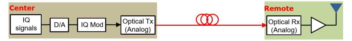
No latency; no synchronization and jitter; co-transmission; better cooperation; low power and weight at RRH
