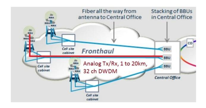
Moving RF Front-End circuitry and/or beamforming circuits to the remote BBU.
