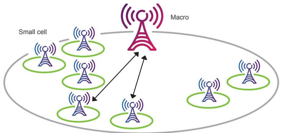
Figure 1: The macro layer and a small-cell cluster
