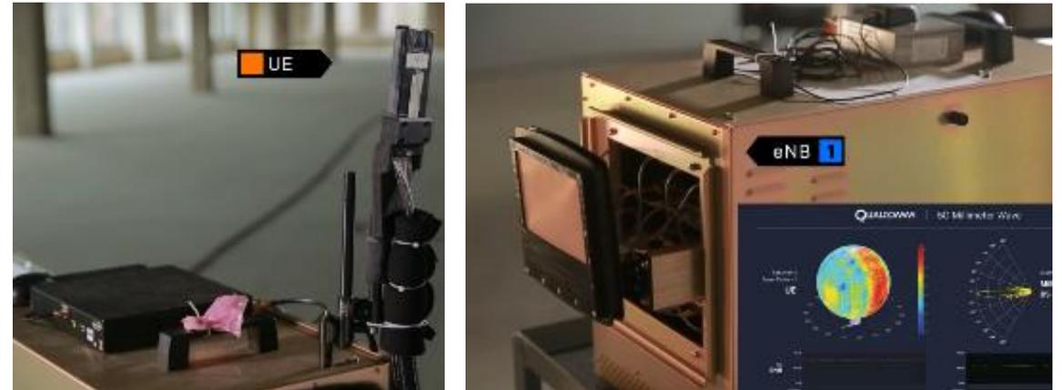
End-to-end system operating at 28 GHz, demonstrating beam forming and scanning to address non-line-of-sight scenarios, improve indoor/outdoor range, and provide robust mobility
